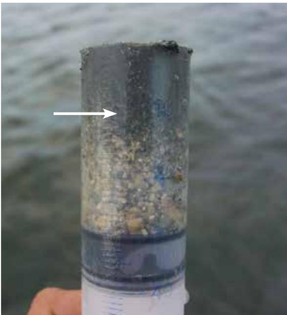
Figure 2. Sediment corer used to quantify oxygen penetration depth. Consistently darker sediment indicates anoxic sediment, as indicated by a white arrow.
