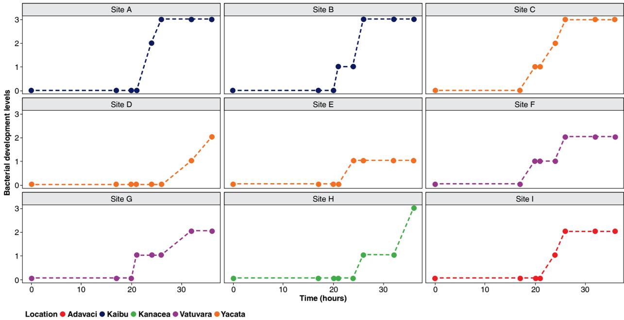
**Figure 5.** Colour development in the hydrogen sulphide water tests at each site surveyed across the islands. Y-axis represents bacterial development levels denoted on a scale 0–3, where 0=clear water (no bacterial development), 1=water turns light grey (indicating presence of bacteria), 2=water turns dark grey (indicating moderate level of bacteria) and 3=water turns black (indicating high level of bacteria).
